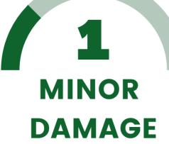
No more than 1 broken window, door or garage door; less than 15% roof cover or wall cladding damage.
